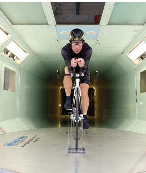
Tour de France champion Lance Armstrong testing a bicycle at the San Diego Air & Space Technology Low Speed Wind Tunnel in November 2008. Armstrong's clothing, helmet, posture, and hand position are also aerodynamically optimized.
